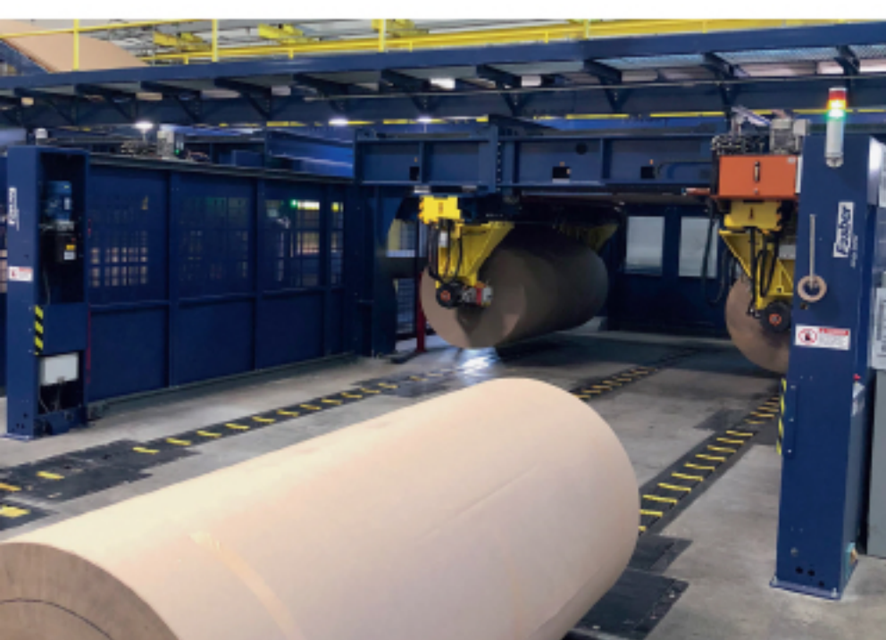
Fosber's Link M3 roll stand/splicers can change paper rolls in less than 120 seconds.
