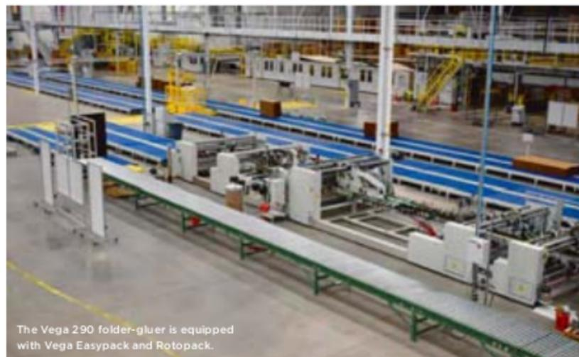
The Vega 290 folder-gluer is equipped with Vega Easypack and Rotopack.
