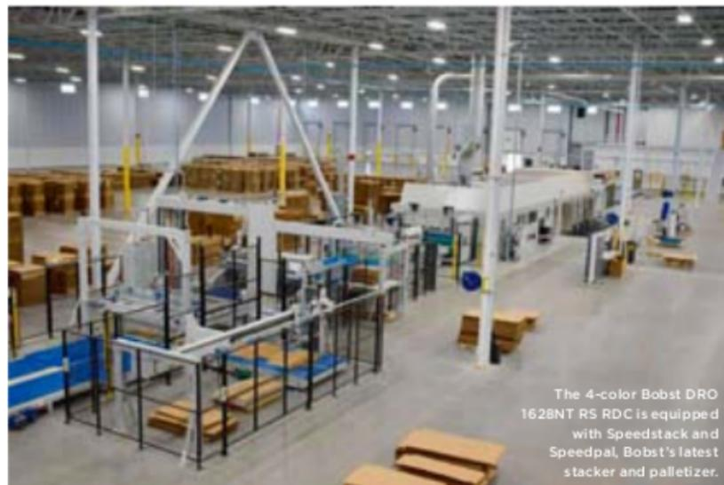
The 4-color Bobst DRO 1628NT RS RDC is equipped with Speedstack and Speedpal, Bobst's latest stacker and palletizer.
